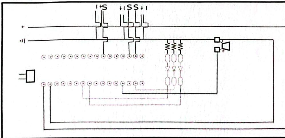
**Figure 14.** Schematic diagram of the transmitter.
