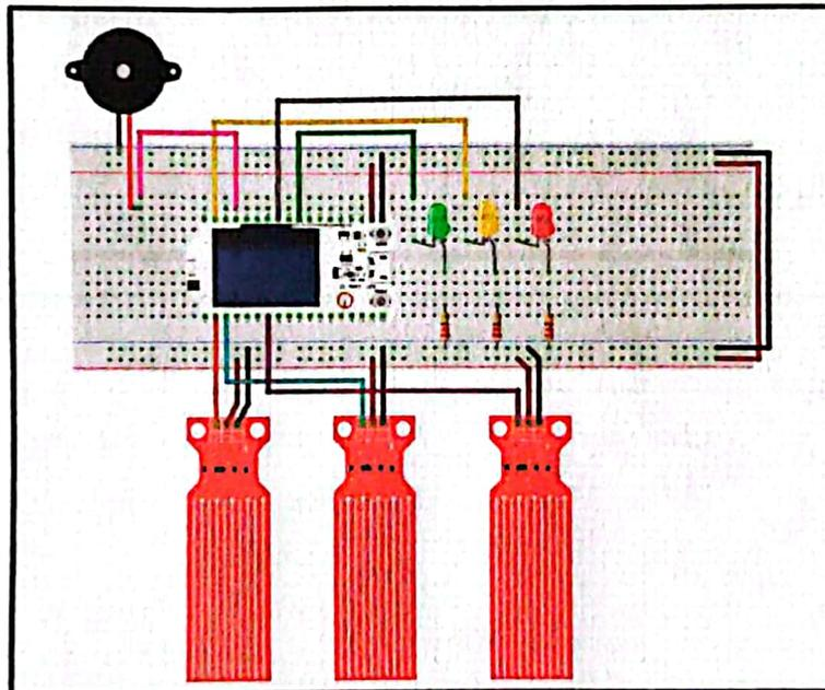
*Figure 13. Structure/ Design of the water level monitoring system.*
